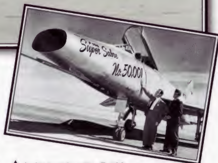
▲ In its heyday, the F-100 equipped 16 full USAF wings, assuming a fighter-bomber role as faster interceptor types became available. It was the USAF's first fighter to reach Mach 1 in level flight.
